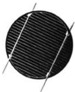
Figure 2. Typical solar cell showing electrode grid pattern
